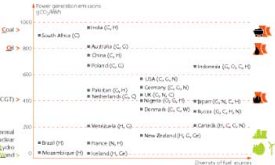
Figure 4: CO 2 intensity of various types of power generation and the current intensity in a range of countries (year 2000 data, electricity and heat generation including auto producers). Fuel sources for each country are ranked in order of importance, with those contributing less than 10% not identified.
